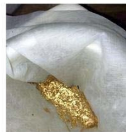
2.c. Extracting Gold: gold residue on filter
